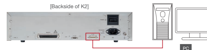
K2 is connected to the PC using a dedicated cable to give high reliability. A PCI express interface card is fitted to the PC.
